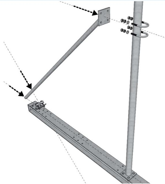
**i** Attach lower part of the central strut to the **GR120-15-P50** supports using 2x M12x100mm bolts
