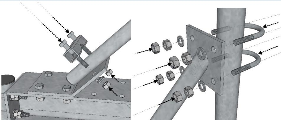
**i** Install on the main pole **GR120-15-P51** connection for the side strut support.
